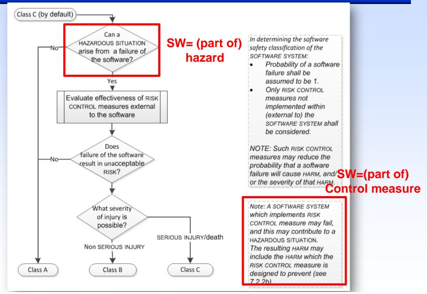
NOTE 1 External RISK CONTROL measures can be hardware, an independent SOFTWARE SYSTEM, health care procedures, or other means to minimize that software can contribute to a HAZARDOUS SITUATION.
